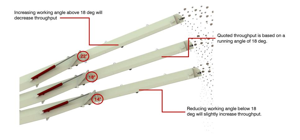
Feed method, material characteristics and environmental conditions can affect throughput, overall performance and maximum working angle.
